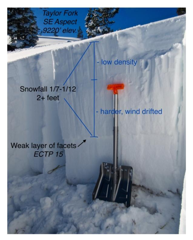
A thin weak layer of facets that formed during cold temperatures are buried by last week's 2+ feet of snowfall. We found unstable test results in this pit, and the poor structure makes avalanches possible to trigger on this layer. Photo: GNFAC
