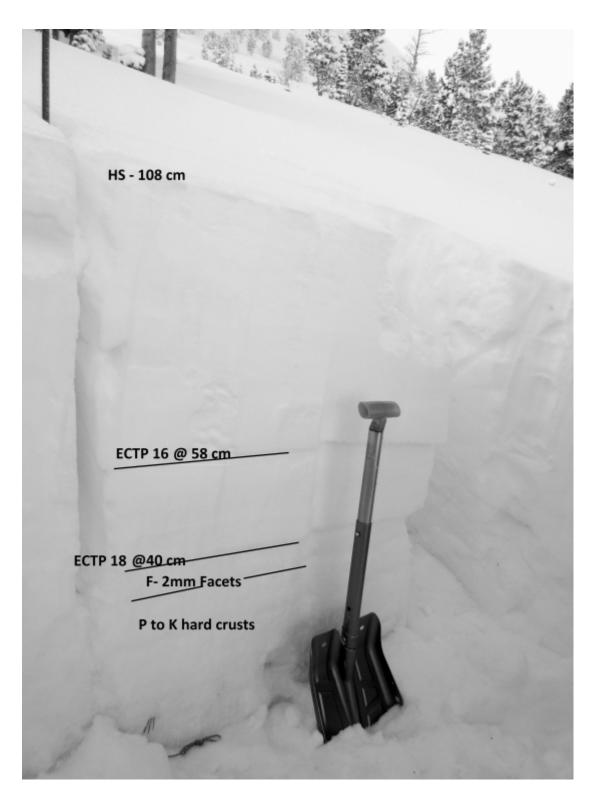
Snowpit from ~9400', northeast aspect, 24 degree slope at the Yellowstone Club in the Northern Madison Range. Weak faceted layers below the previous week's snowfall propagated fractures in stability tests. This shows a poor snowpack structure, and cold temperatures are making these facets weaker. Photo: GNFAC
