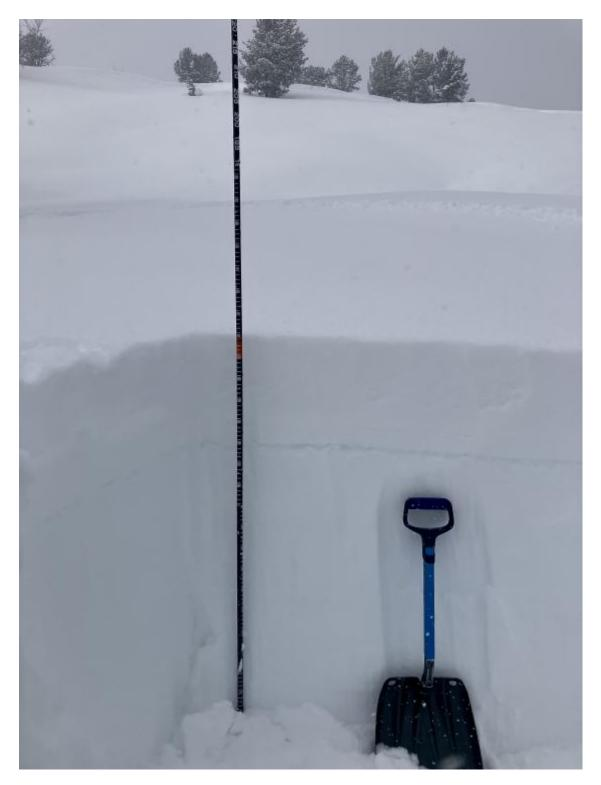
Jan 24, Buck Ridge... We dug on an E facing slope at 9,400'. Snow depth was 155cm (5 feet) and we had an ECTN12 on the surface hoar layer 10" down. Photo GNFAC
