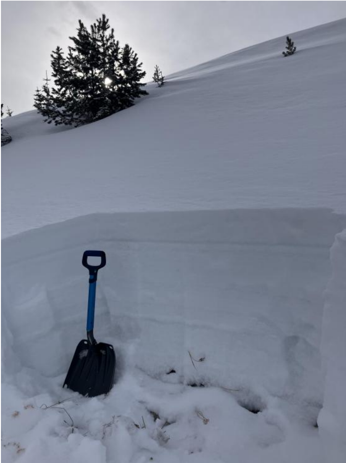
Snowpit in Second Yellow Mule. The gray line above the shovel is a layer of well-preserved buried surface hoar 12-16mm in size. Photo: GNFAC
