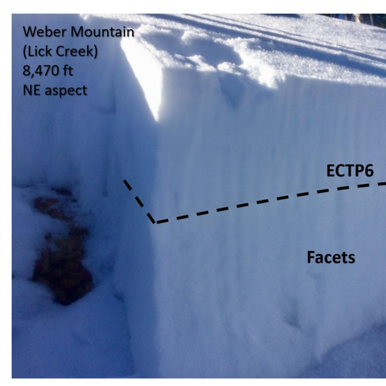
Skiers observed collapsing on Weber Mountain near Lick Creek in Hyalite. They dug a pit and found poor structure with a thin, faceted snowpack and got poor stability test results, with ECTP6 failing on a thick layer of facets. Photo: M. Talty
